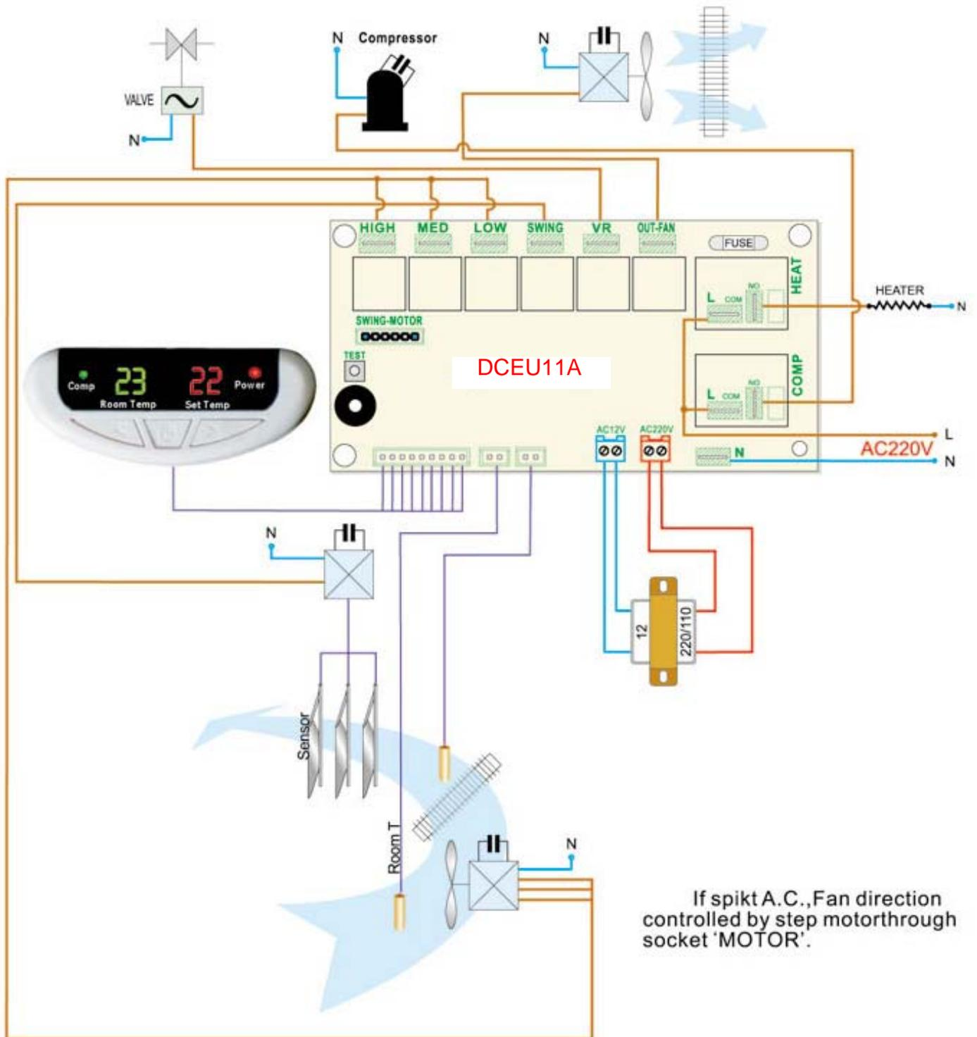
If spikt A.C., Fan direction controlled by step motorthrough socket 'MOTOR'.
